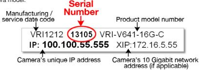
2) Where to physically locate the serial number label on your Phantom camera The location will also vary depending on camera model. Some common examples are pictured here.
