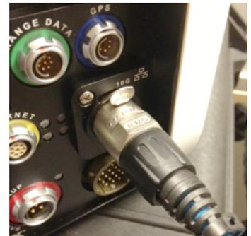
Ruggedized Ethernet Connector installed on Cat 6a cable in Phantom V1610's RJ45 port
